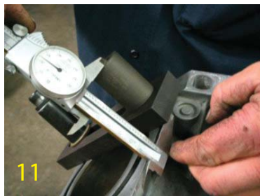
11 measure the assembled thickness of the drill plate and the second drill bushing. Add both measurements together.
