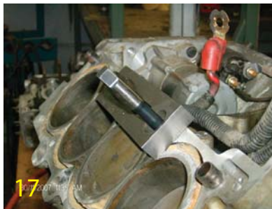
17 For extra deep holes, remove the tap alignment bushing and continue tapping to depth.
