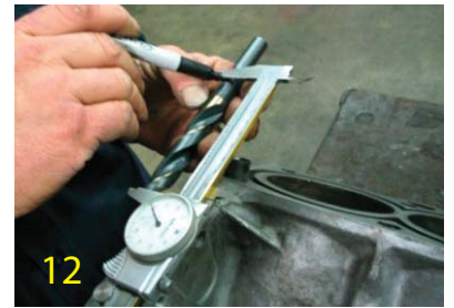
12 Mark the 39/64" drill bit the same way as the first drill bit.
