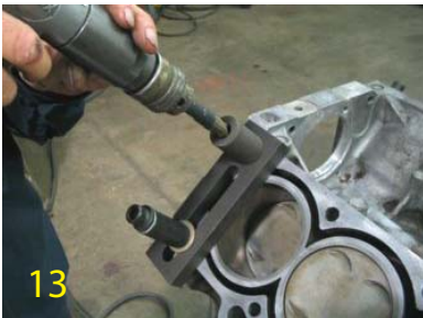
13 Now drill down to the starting point of the original threads. This creates clearance for the tap so you will only thread the bottom of the hole.
