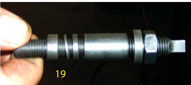
19 The deep reach installation tool comes with a threaded stud, drive nut, surface washer, bottom 1/4" threaded spacer, 1", 1/2", 1/8" and 1/16" thick spacers that can be stacked to allow installation depths adjustable in 1/16" increments ranging from flush to 2 3/16" below the surface.
