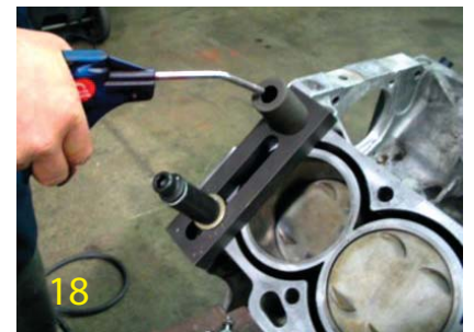
18 Remove the tap and blow out the shavings.
