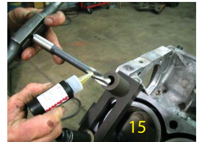
15 Install the FTCM4TG tap bushing and apply a liberal amount of the L852 tapping fluid to the tap.
