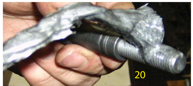
20 After stacking the desired sizes of spacers including the bottom threaded spacer to equal the right deep recess, Tighten the bottom threaded spacer upward until all spacers are compressed against the surface washer. Next apply a small amount of anti-seize the bottom end of the threads to prevent the thread locker from getting between the insert and the stud.
