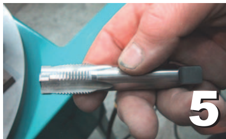
The Tap (FT5RPLT) is piloted to assure proper alignment.
