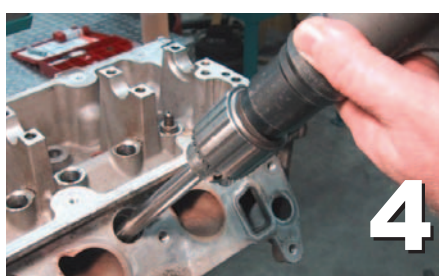
Bore Out the hole to 41/64".
