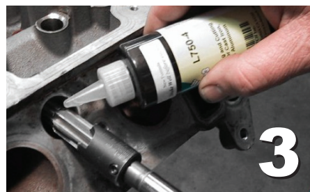
Apply L750 Cutting Fluid to the Core Drill. (Shake well before using)
