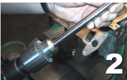
Chuck the Core Drill shaft into a 1/2" drill.
