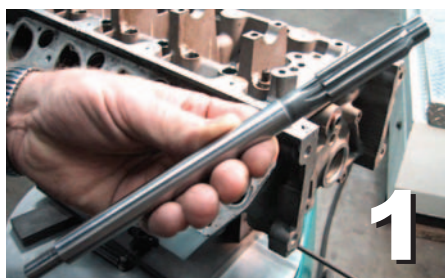
The piloted Core Drill (FT4164CD) oversized the hole for the tap.
